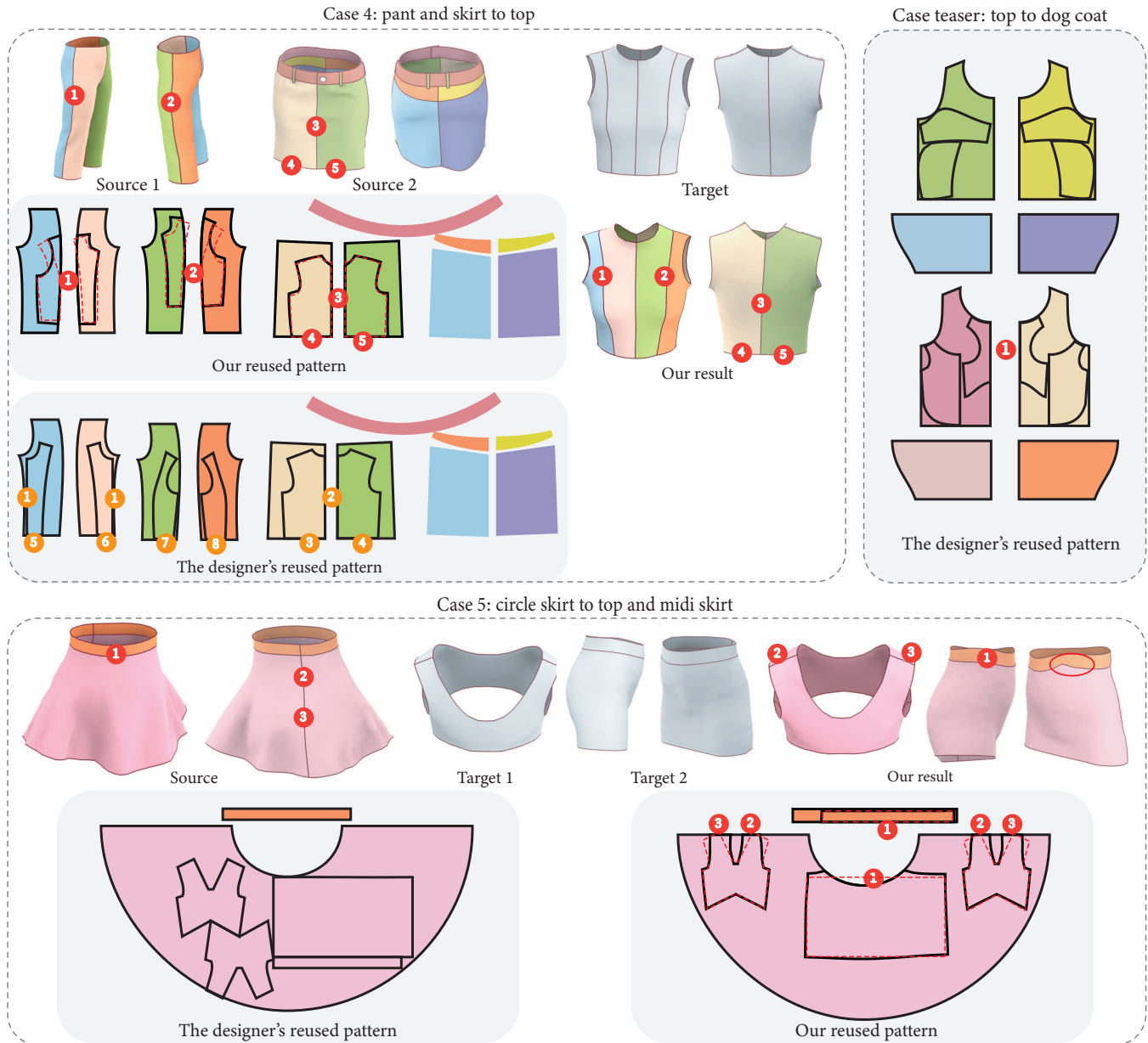
Fig. 10. Results and comparison to manual designs. In Case 4, two sources are combined into one target, while in Case 5, a single source is used to form two targets. Note how Case 5 demonstrates significant reuse of seams thanks to deformation of the target panels. While these deformations change the shape of the top a little, we highlight a stronger deformation along the waist of the skirt. Case 4 also introduces deformations for the panels cut on the pants, yet these deformations are difficult to notice in the final 3D garment. We also provide the reused patterns produced by a professional fashion designer on these cases, as well as on the case shown in Figure 1. In particular, the designer took similar decisions to ours in Case 4, while they did not reuse any seam or hem in Case 5. Note that while reusing seam (1) of Case 4 would require deforming the panels, the designer did not depict that deformation.
