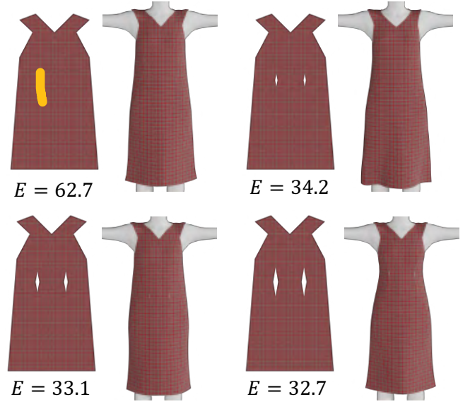
Figure 2: Double-pointed dart design on a dress during the optimization of dart shape ( w, h ). We report the Energy E at the k iterations where k = 0, 5, 15, 20 (converged). The yellow stroke on the first pattern indicates the user's input.
