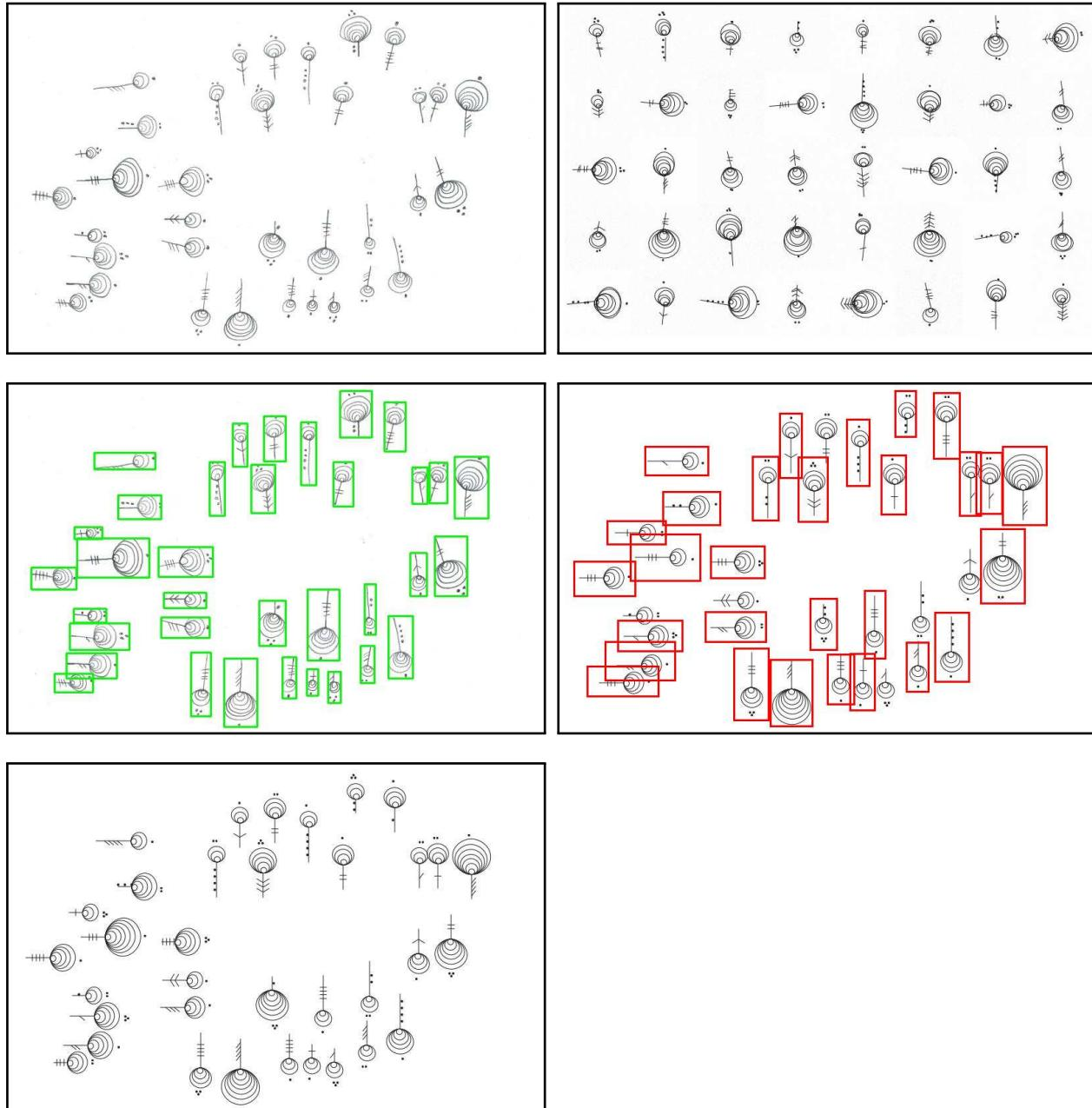
Figure 11: Results for the *Lollipop* design. Input image (top left), sampled glyphs from the training dataset (top right), detected glyphs (center left, green boxes indicate True Positive detection and red boxes indicate False Positive detection), reconstruction from the estimated parameter values (center right, red outlines indicate glyphs for which one or several parameter values are erroneous), reconstruction from the ground truth parameter values (bottom left).
